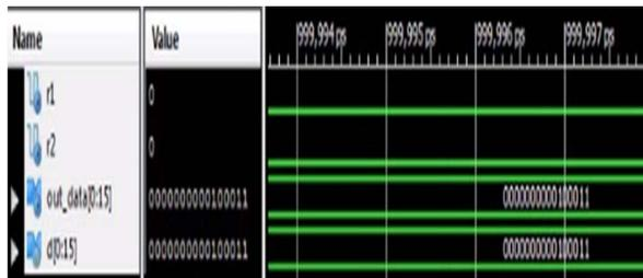
Fig. 3. Simulation results for OLS codes when  $r_1r_2=00$
