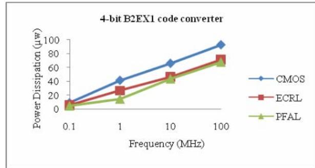
Fig.9. Average power dissipation of binary to excess-1 code converter at different frequencies
