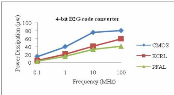
Fig.7. Average power dissipation of Binary to Gray code converter at different frequencies
