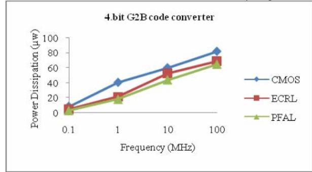
Fig.8. Average power dissipation of Gray to Binary code converter at different frequencies
