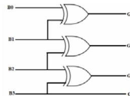
Fig.4. 4-bit Binary to Gray code Converter
