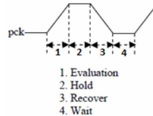
Fig.3. Phases in Adiabatic power supply
