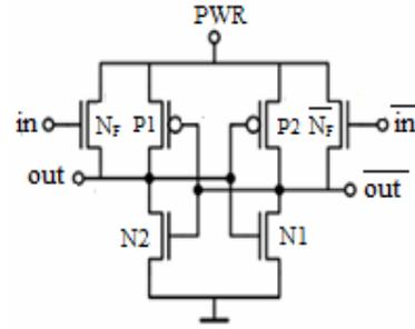
Fig.2. Basic PFAL inverter/buffer
