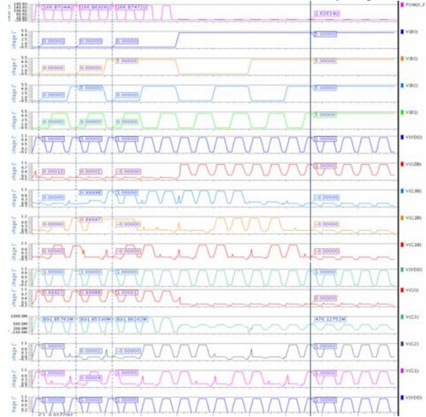
Fig.8.Simulation waveform of 4-bit PFAL Binary to Gray Code Converter
