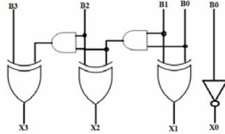
Fig.6. 4-bit Binary to Excess-1 code converter
