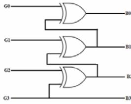
Fig.5. 4-bit Gray to Binary code converter
