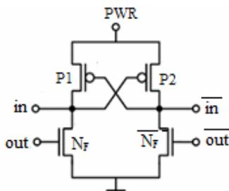
Fig.1. Basic ECRL inverter/buffer
