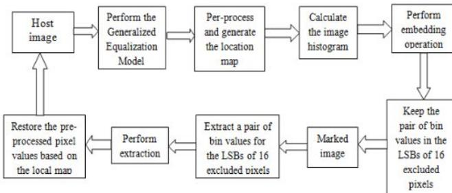
Figure 2. Block diagram of the proposed RDH algorithm
