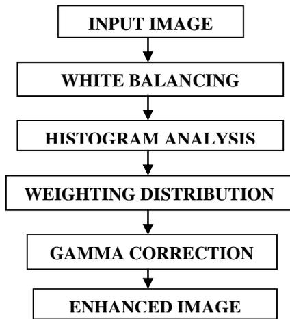
Figure1. Block diagram of generalized equalization model
