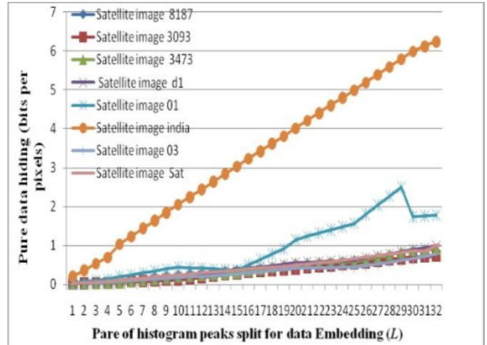
Figure 5. The data hiding rates generally increase with the number of histogram peaks used for data embedding (for 8 Getty satellite images)
