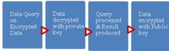
Figure 4: Query processing in Traditional Encryption System
