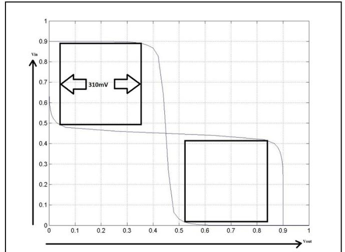
Fig.10 Butterfly curve for 6T SRAM cell
