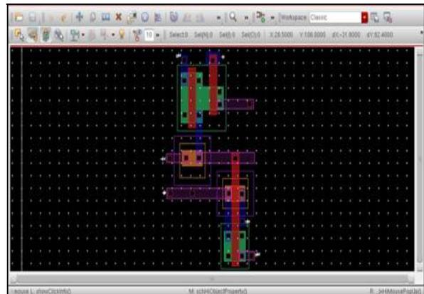
Fig.12 Layout of standard 5T (WM max)
