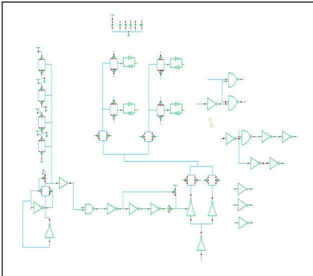
Fig.4 Schematic of write assist Circuit.
