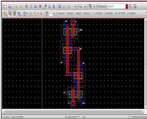
Fig.13 Layout of standard 6T
