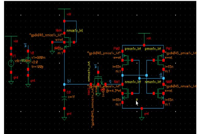
Fig.6 Schematic of 5T SRAM cell
