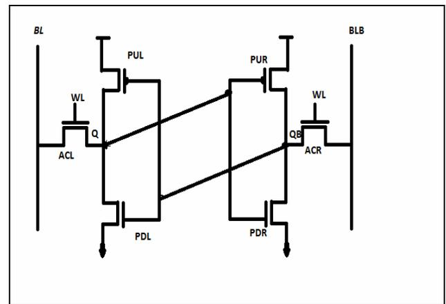
Fig.1. The standard 6T SRAM cell
