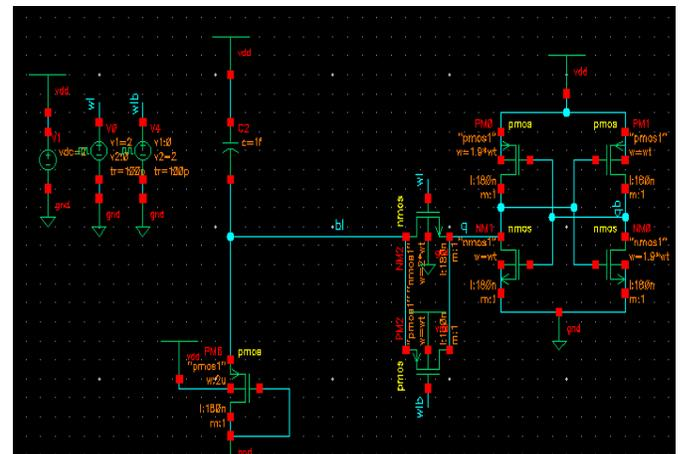
Fig.7 Schematic of 6T SRAM cell using TG
