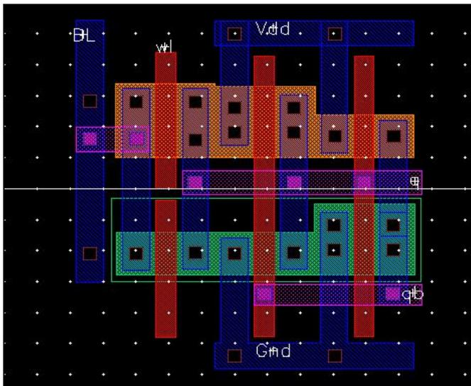
Fig.14 LAYOUT OF 6T USING TGS
