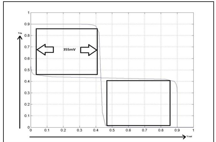
Fig.11 Butterfly curve for 6T SRAM cell using TG
