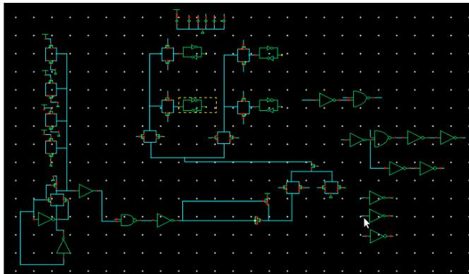
Fig.5 Schematic of proposed write assist Circuit.
