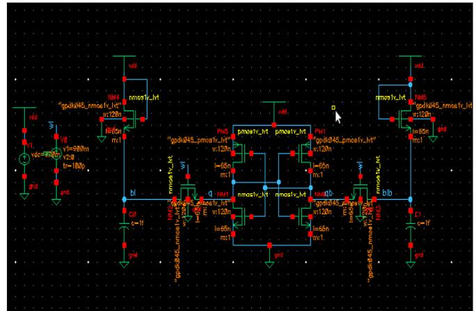
Fig.5 Schematic of 6T SRAM cell
