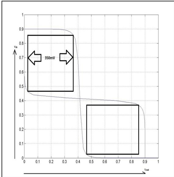
Fig.9 Butterfly curve for 5T (RSNM max)
