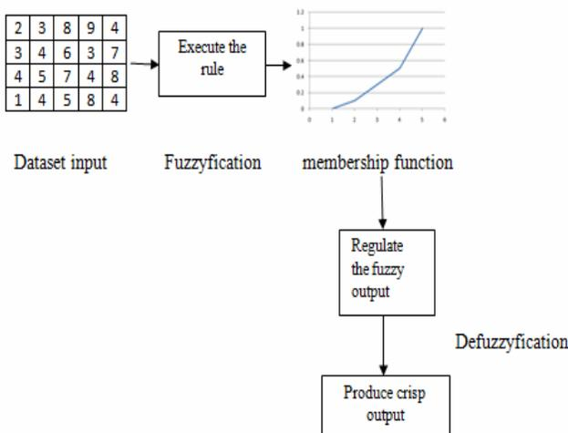
Figure 4. Overall structure of fuzzy system.
