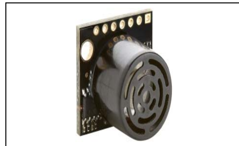
Figure 7. Maxbotix sonar used in experiments.
