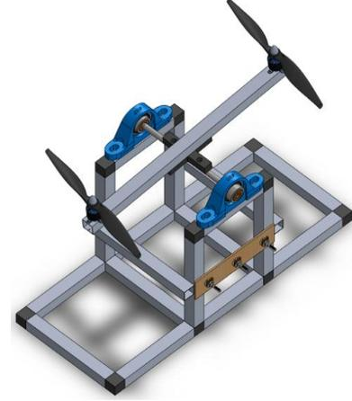
Fig. 2. Half-quadcopter experimental setup layout
