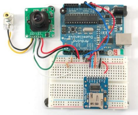
Fig 3. Arduino board with camera and sd card.
