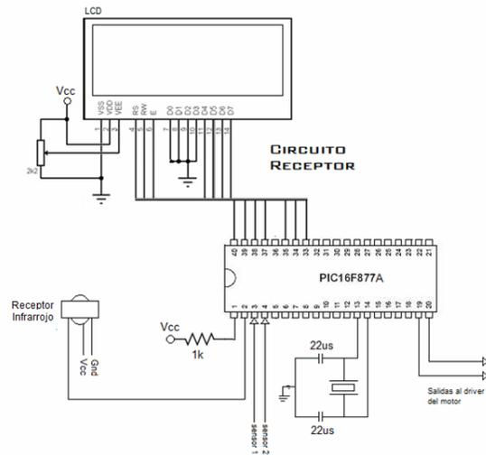
Figure 5 circuit receiver
