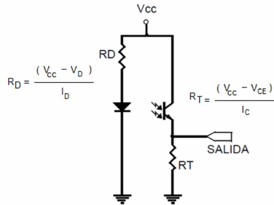
Figure 8 Configuration used in the design of a sensor Encoder of a single contact
