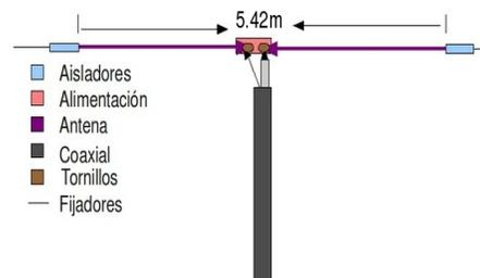
Figure 1 Dipole antenna
