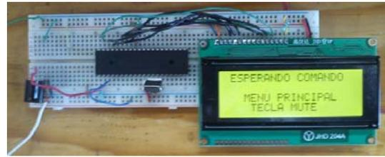
Figure 11 Receiver circuit complete with LCD showing message
