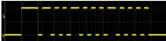
Figure 10 Signal corresponding to the 0 key
