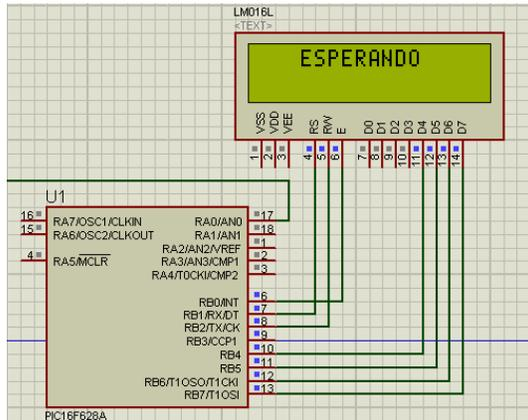
Figure 7. Circuit LCD Operation
