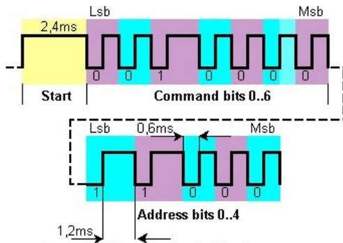
Figure 4 Signal delivered by the remote control
