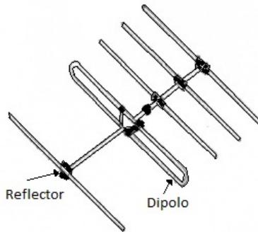
Figure 2. Yagi Antenna
