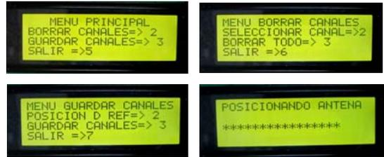
Figure 12 Screens showing the different menus. Showing different messages presented on the LCD for the receiver circuit which correspond to different circuit functions.
