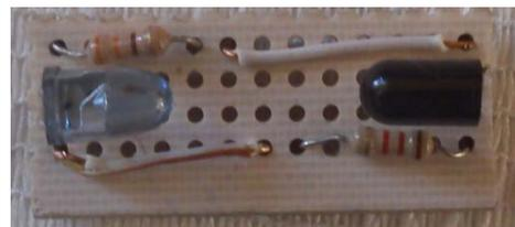
Figure 13 already mounted physical sensor using a Emitting diode and a phototransistor
