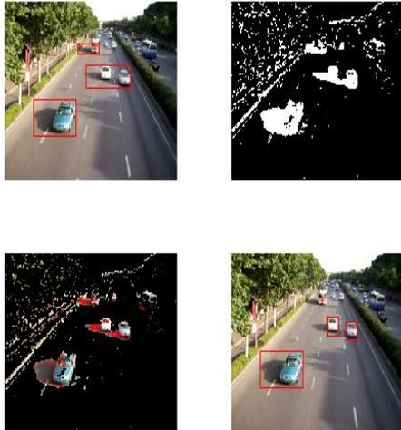
Fig. 2. Output for Frame # 128 A) showing clutter effect B) foreground pixel separation using GMM C) shadow pixels D) clear segmentation of objects
