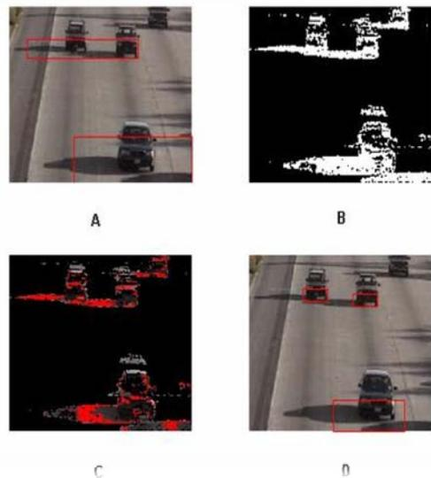
Fig. 1. Output for Frame # 74 A) showing clutter effect B) foreground pixel separation using GMM C) shadow pixels D) clear segmentation of objects.
