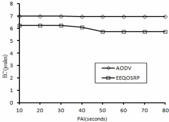
**Figure 4 shows EC with PAI for Existing and Proposed Model**
