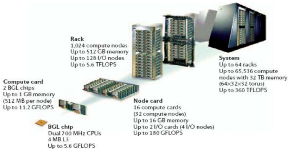
Fig. 4.1. The Blue Gene/L supercomputer architecture
