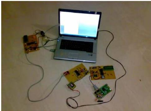
As depicted in fig.1 an advanced controlling system using zigbee is implemented for controlling labs PCs and other equipment like lights, fans air conditioners etc.
