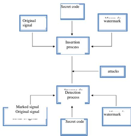
Fig 2. Generic diagram of digital watermarking.
