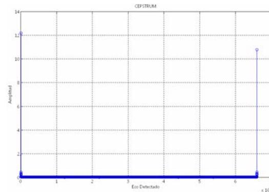
Fig 4. Graph showing the detection of delayed samples in an audio clip.
