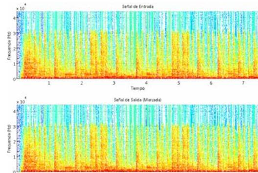
Fig. 3 Frequency spectrum of an audio clip original and marked
