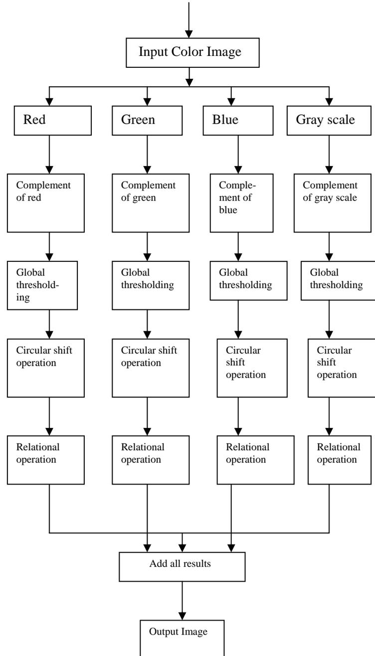
Fig.1 The Block diagram of the proposed method
