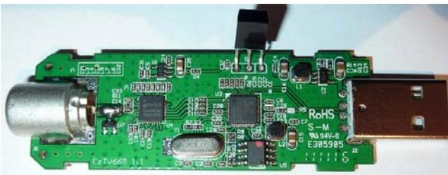
Figure 9. RTL-SDR hardware
