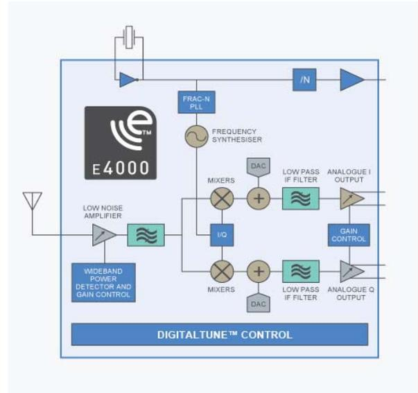
Figure 10. Elonics E4000 tuner chip block
