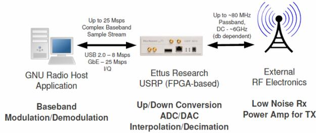
Figure 6. Control flow in systems with USRP
