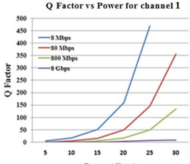
Fig 6. Q factor vs Transmitted Powers for different bit rates.
