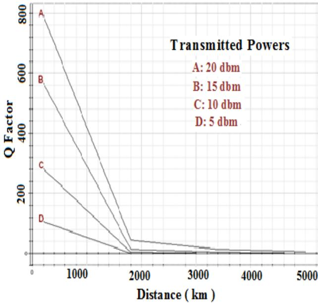
Fig.5. Q Factor vs link distance for different transmitted powers.
