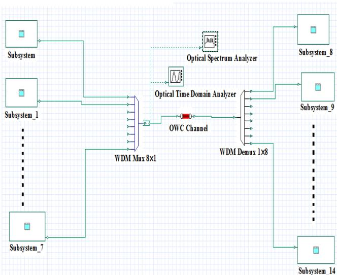
Fig.4. Simulation Model of 8-Channel WDM System for intersatellite optical link.
