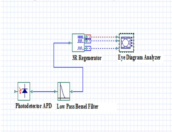
Fig .3(b). The structure of a sub system at receiver side
