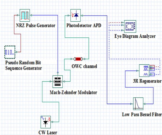
Fig 2. IsOWC simplex design model
