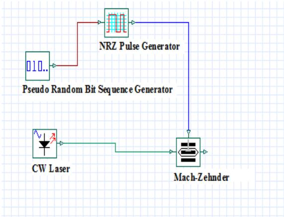
Fig .3(a). The structure of a sub system at transmitter side
