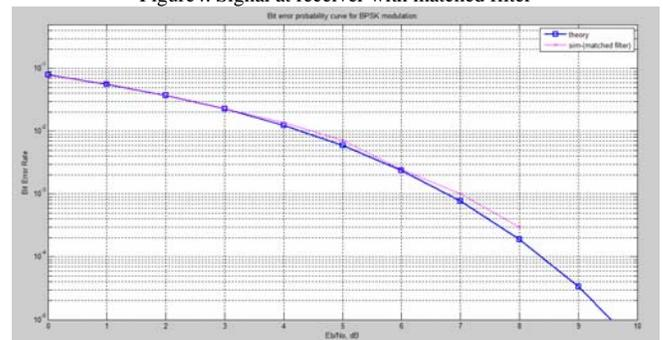
Figure5. Average bit error rate with matched filter
