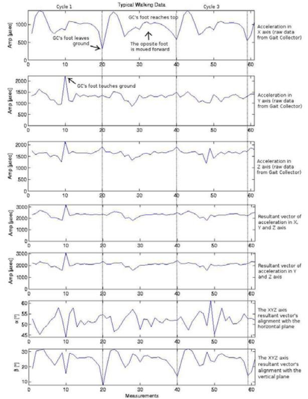
Figure 11: Shows the data gathered from the Gait Collector over three gait cycles.
