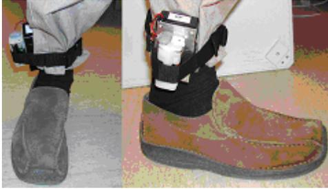
Figure 5: The Gait Collector attached to a person’s leg in its ideal position just above the right foot’s ankle
