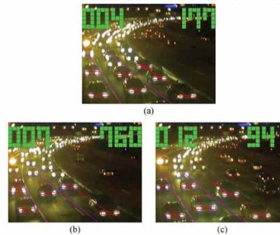
Fig.5 Results of vehicle detection and classification for a congested highway traffic scene under a light environmental illumination condition.
